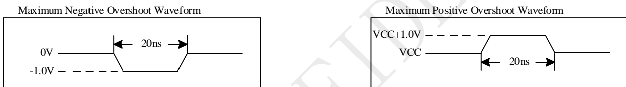
Figure 5-2 Input Test Waveforms and Measurement Level
