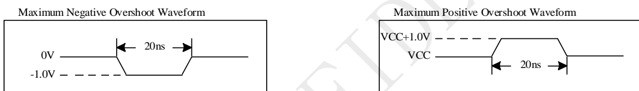
Figure 5-1 Maximum Overshoot Waveform
