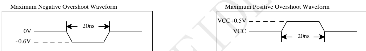
Figure 5-1 Maximum Overshoot Waveform
