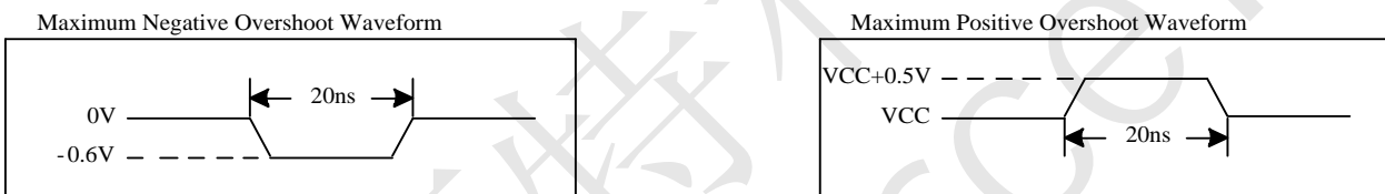
Figure 5-1 Maximum Overshoot Waveform
