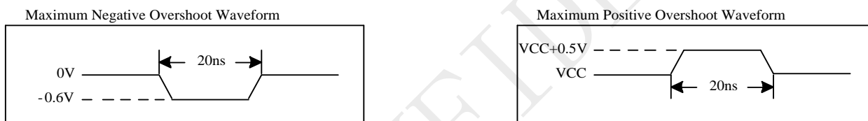
Figure 5-1 Maximum Overshoot Waveform
