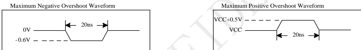
Figure 5-1 Maximum Overshoot Waveform
