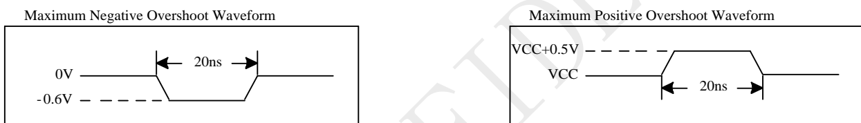
Figure 5-1 Maximum Overshoot Waveform
