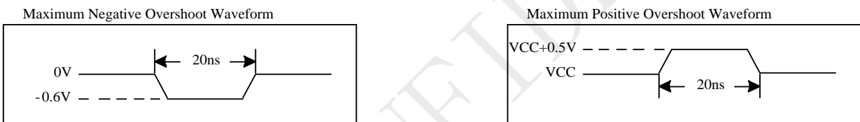
Figure 5-1 Maximum Overshoot Waveform
