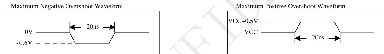
Figure 5-1 Maximum Overshoot Waveform
