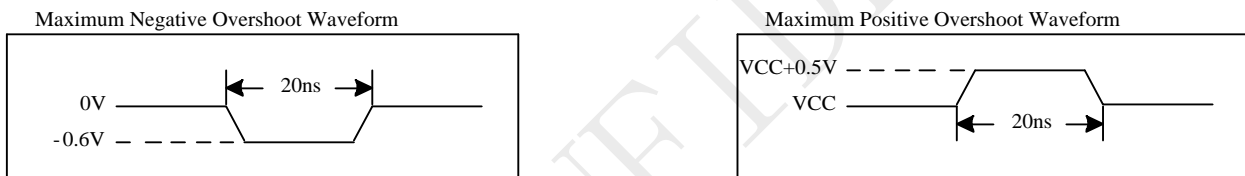
Figure 5-1 Maximum Overshoot Waveform
