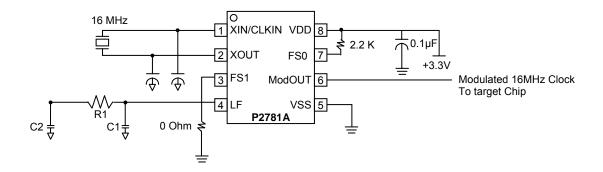
Note: Both logic input pins FS1 and FS0 have to be connected to either VDD or VSS. Do not leave them floating.
