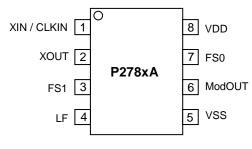
Standard pin Configuration offered in both 8 pin SOIC Packages.
