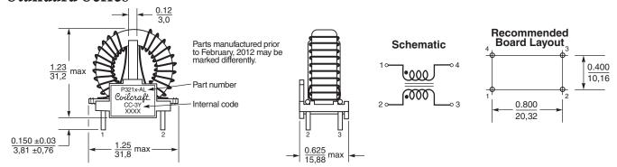
Tin-silver over copper; #16 AWG (0.051"/1,29 mm) except Terminations: P3217-A, which has #18 AWG (0.040"/1,02 mm).
