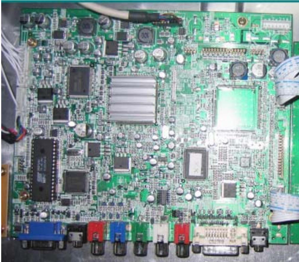
Printed Circuit Audio Board , In bom we call it Emulation board subassembly
