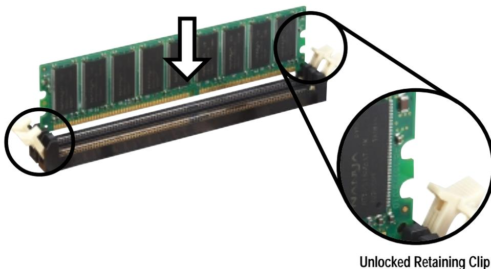
3. Firmly insert the DIMM into the socket until the retaining clips snap back in place and the DIMM is properly seated.
