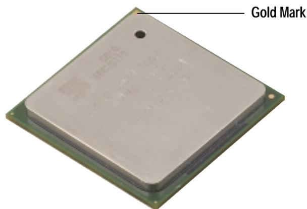
Note in the illustration that the CPU has a gold triangular mark on one corner. This mark indicates the processor Pin 1 that should match a specific corner of the CPU socket.
