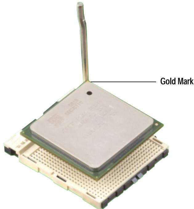
5. When the CPU is in place, press it firmly on the socket while you push down the socket lever to secure the CPU. The lever clicks on the side tab to indicate that it is locked.
