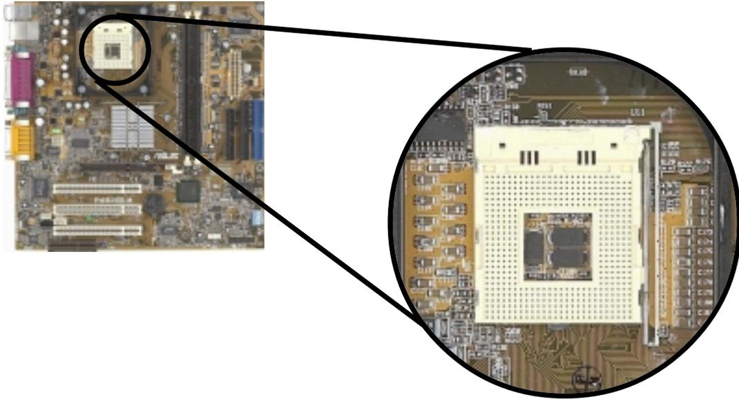
2. Unlock the socket by pressing the lever sideways, then lift it up to a 90°-100° angle.
