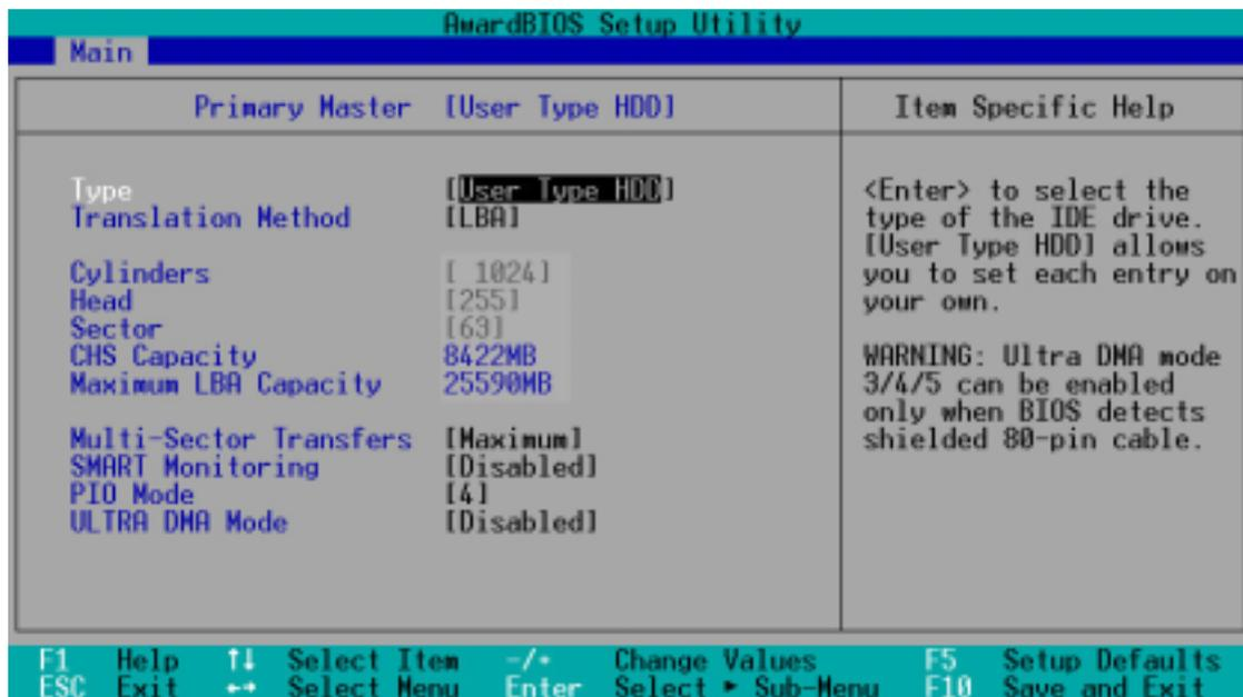
Manually enter the number of cylinders, heads and sectors per track for the drive. Refer to the drive documentation or on the drive label for this information.
