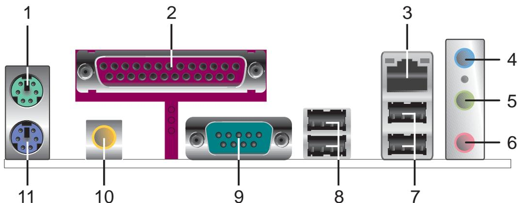
1. **PS/2 mouse port.** This green 6-pin connector is for a PS/2 mouse.
