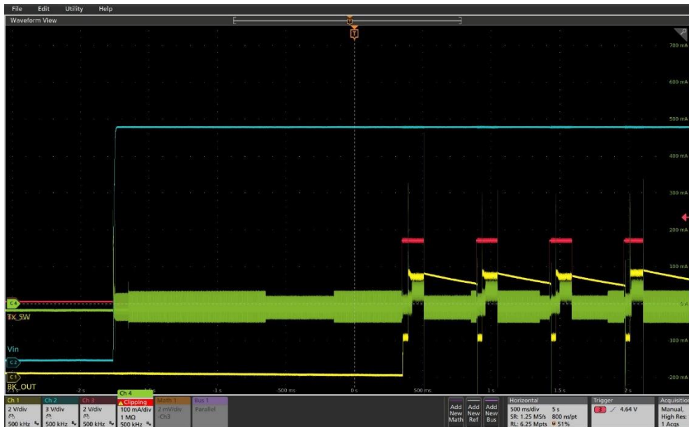
Figure 9. 19V Fixed Voltage Adaptor Start-up: Ch1 = VBRIDGE, Ch2 = V_{in} , Ch3 = GPIO_B4, Ch4 = i_{in}
