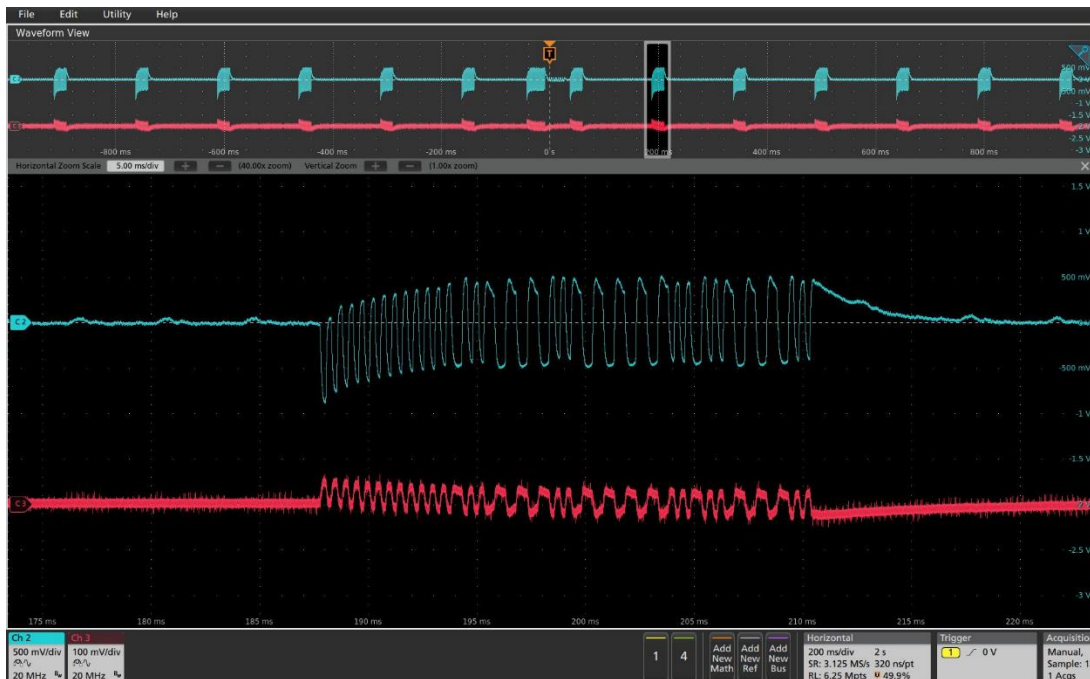
Figure 7. Voltage and Current Signal for Demodulation: Ch2 = VSNS, Ch3 = ISNS_IN
