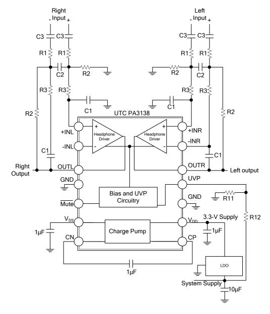
R1=15k $\Omega$ , R2=30k $\Omega$ , R3=43k $\Omega$ , C1=47pF, C2=180pF
