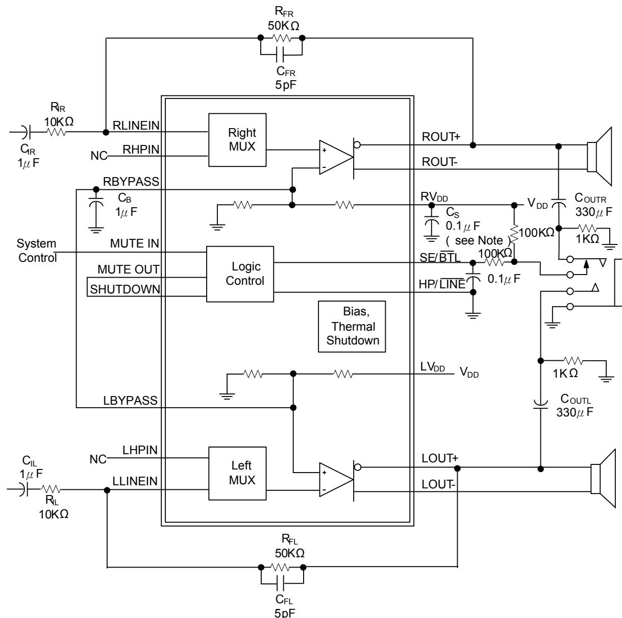
Note: 0.1  $\mu$  F ceramic capacitor should be placed as close as possible to the IC. For filtering lower frequency noise signals, a larger aluminum electrolytic capacitor of 10  $\mu$ F or greater should be placed near the audio power amplifier.
