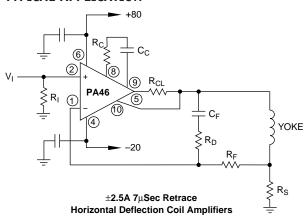
Horizontal deflection amplifiers require both high speed and low distortion. The speed at which current can be changed in a deflection coil is a function of the voltage available from the op amp. In this application an 80 volt power supply is used for the retrace polarity to provide a 7  $\mu Sec$  retrace time, half of which is required for amplifier slewing. This circuit can perform 15.75 KHz deflection in up to  $50\mu H$  coils at up to 5A p-p.
