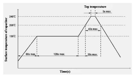
Recommended curve for lead free soldering is as following:
