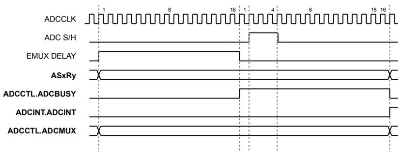
**Figure 17-8. ASxSy Sample with ASxSy.EMUXS = 01b and ASxSy.DELAY = 11b**
