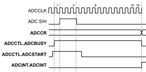
**Figure 17-3. ADC Conversion (Repeat Mode)**
