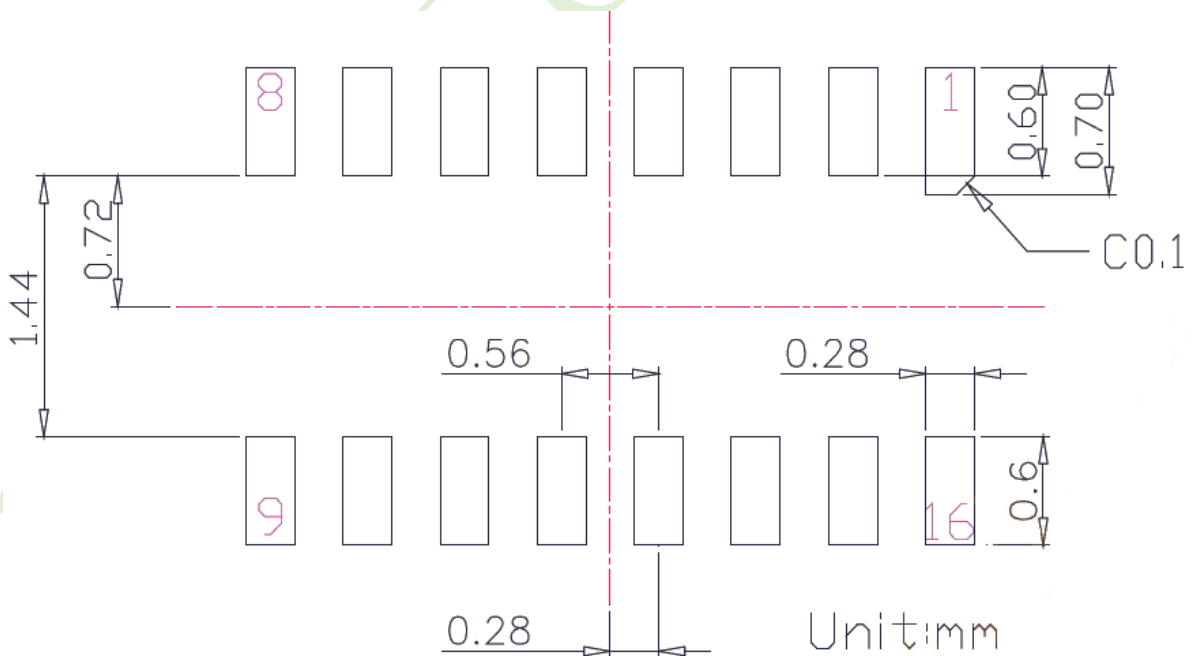
Figure 4. Recommend Layout PCB
