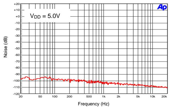
**Performance Characteristics** (@ $T_A = +25^\circ\text{C}$ ,  $V_{DD} = 5\text{V}$ , Gain = 18dB,  $R_L = L(33\mu\text{H}) + R + L(33\mu\text{H})$ , unless otherwise specified.)
