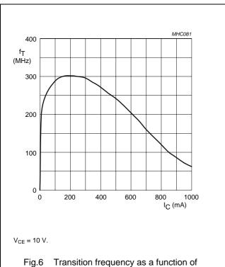
Fig.6 Transition frequency as a function of collector current.
