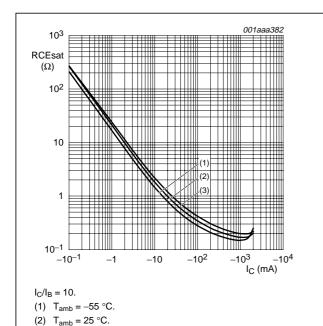
Fig.11 Equivalent on-resistance as a function of collector current; typical values.
