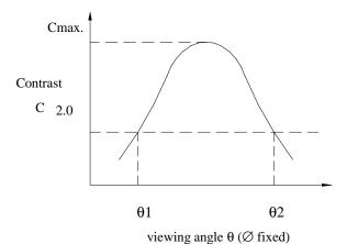
Note: Optimum viewing angle with the naked eye and viewing angle  $\theta$  at
