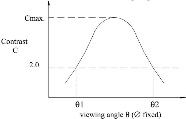
Note : Optimum viewing angle with the naked eye and viewing angle  $\theta$  at Cmax. Above are not always the
