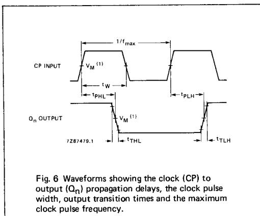
Fig. 6 Waveforms showing the clock (CP) to output ( $O_n$ ) propagation delays, the clock pulse width, output transition times and the maximum clock pulse frequency.
