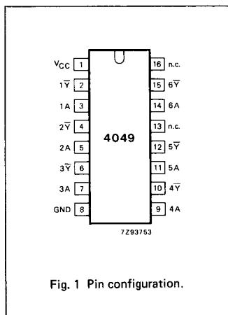
Fig. 1 Pin configuration.
