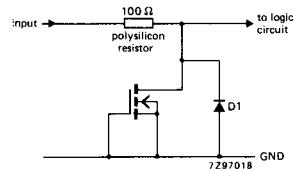
Fig. 5 Input protection for HC4049.
