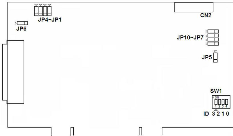
Figure 3.2: Location of Jumpers & DIP Switch
