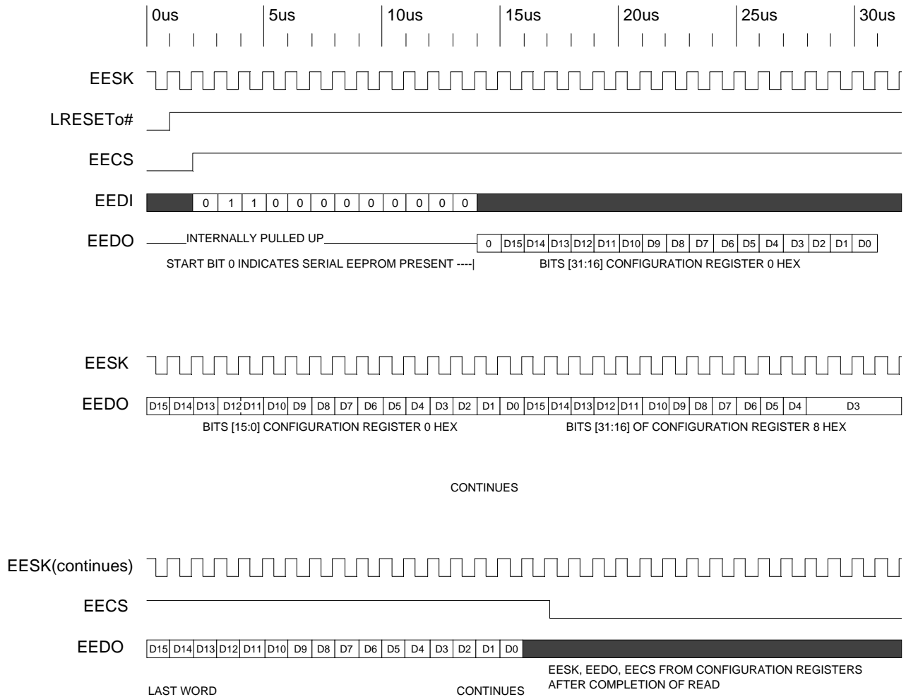
Timing Diagram 4-1. Initialization from Serial EEPROM (2K Bit)
