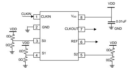
Use either pull-up or pull-down  $0\Omega$  Resistor with [S2:S0] for selection of CLKOUT frequencies.
