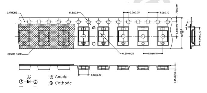
**Note:** The tolerances unless mentioned are ±0.1, unit=mm.
