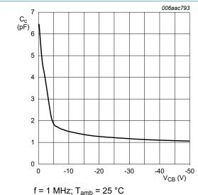
Fig. 7. Collector capacitance as a function of collector- Fig. 8. base voltage; typical values
