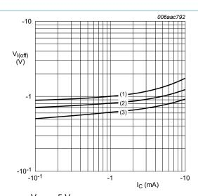
V<sub>CE</sub> = -5 V (1) T<sub>amb</sub> = -40 °C (2) T<sub>amb</sub> = 25 °C
