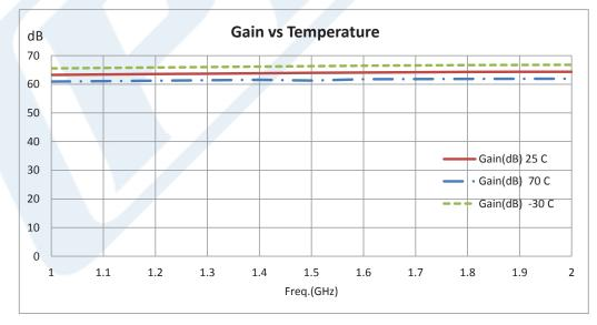
Click the following link (or enter part number in "SEARCH" on website) to obtain additional part information including price, inventory and certifications: 60 dB Gain, 80 mW, 1 GHz to 2 GHz, Limiting Amplifier, -40 to 10 dBm Pin, SMA PE15A6002
