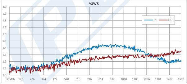
Click the following link (or enter part number in "SEARCH" on website) to obtain additional part information including price, inventory and certifications: 39 dBm IP3, 1.6 dB NF, 23 dBm P1dB, 30 MHz to 1.5 GHz, Low Noise Amplifier, 29 dB Gain, SMA PE15A63003
