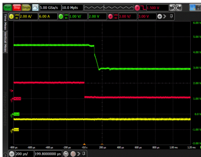
Figure 27. Auto-switch MODE DIV2 to DIV3 transition, I_{OUT} = 1.5A
