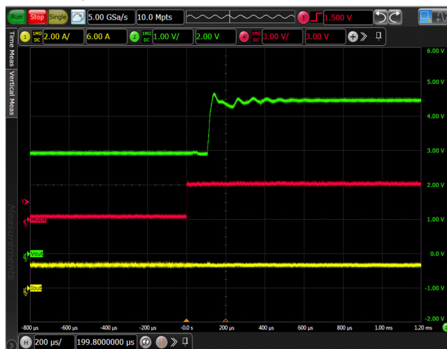
Figure 26. Auto-switch MODE DIV3 to DIV2 transition, I_{OUT} = 1.5A
