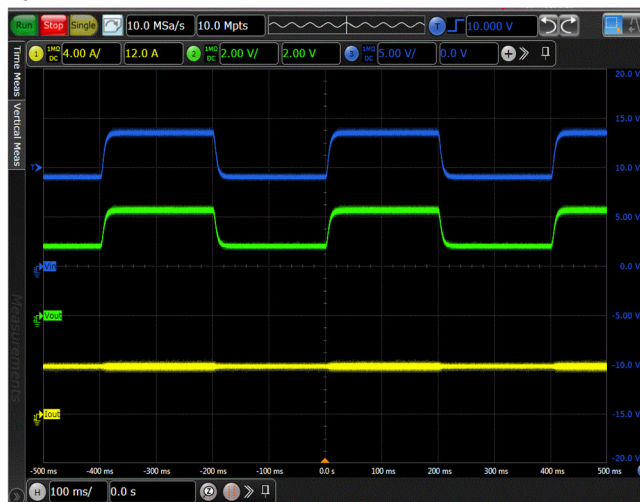
Figure 29. Line transient 9-13.5V I_{LOAD} = 4A DIV3 C_{LOAD} = 100 \mu F
