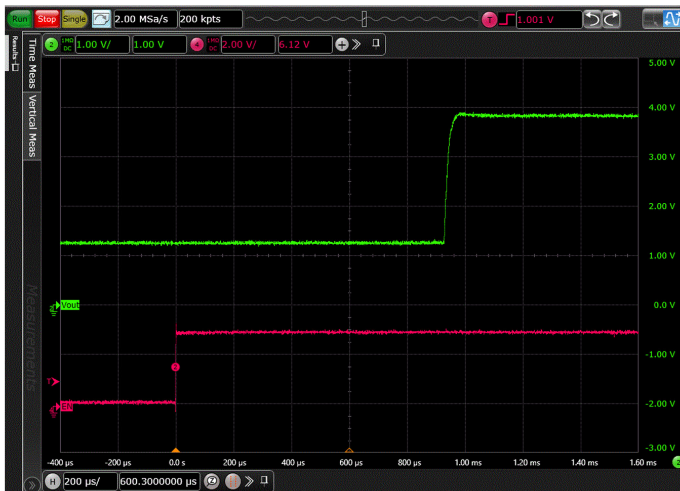
Figure 36. Soft Start into a Pre-charged Load
