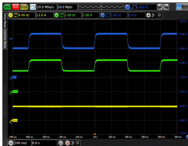
Figure 28. Line transient 6-9V I_{LOAD} = 4A DIV2 C_{LOAD} = 100 \mu F
