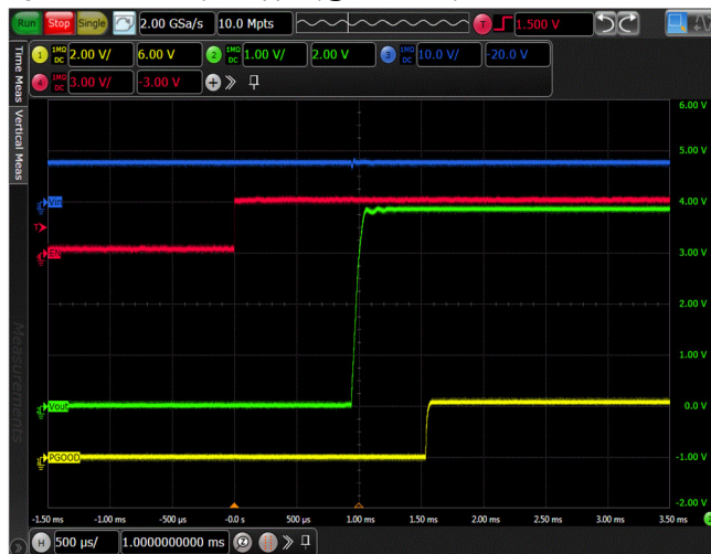
Figure 22. DIV2 Start up, C_{LOAD} = 100 \mu F
