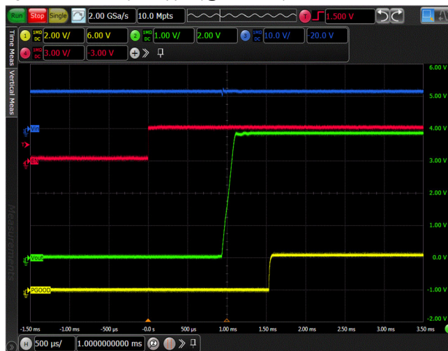
Figure 23. DIV3 Start up, C_{LOAD} = 100 \mu F
