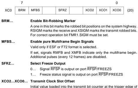
SCLKX when the synchronous pulse on port SYPX is active. Setting of SIC1.SXSC enforces programming the offset values in the range of 0 to 192 bits with XCO0 always cleared.
