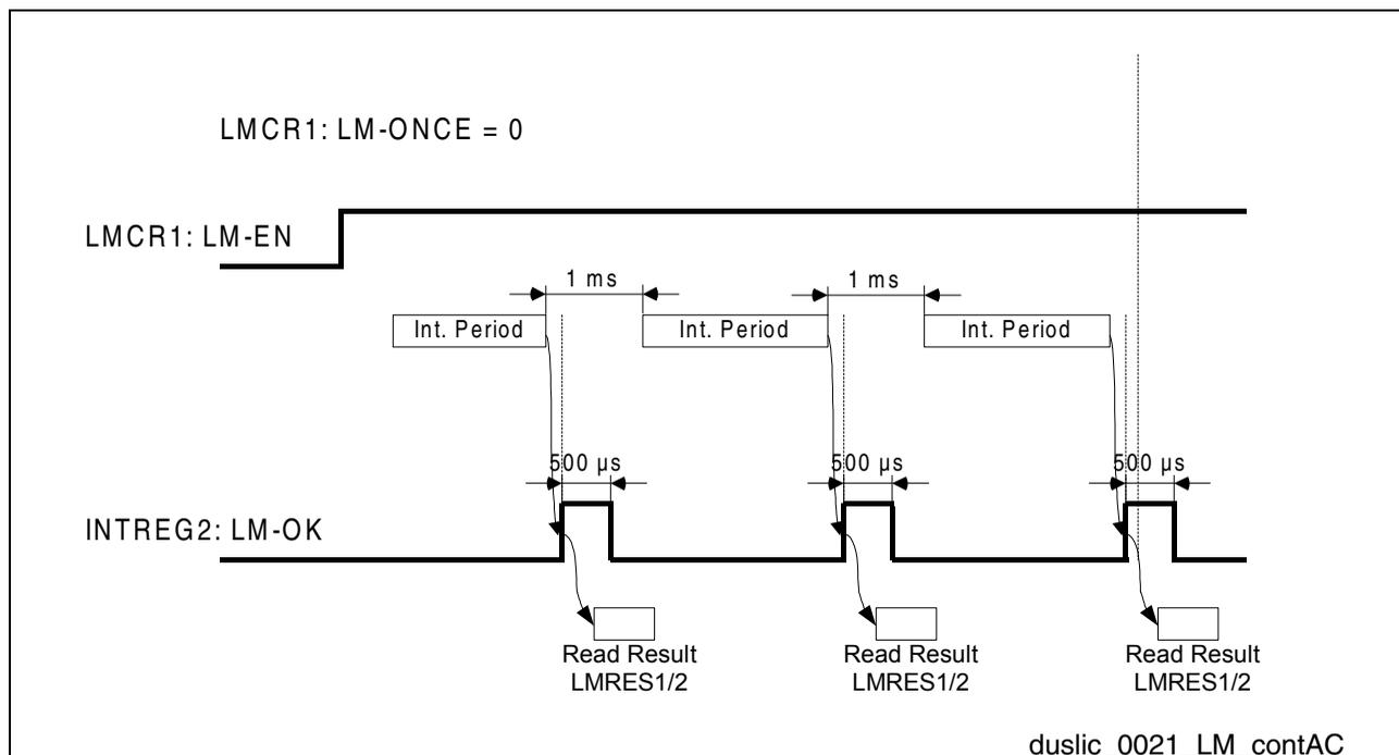
**Figure 43 Continuous Measurement Sequence (AC Level Metering)**
