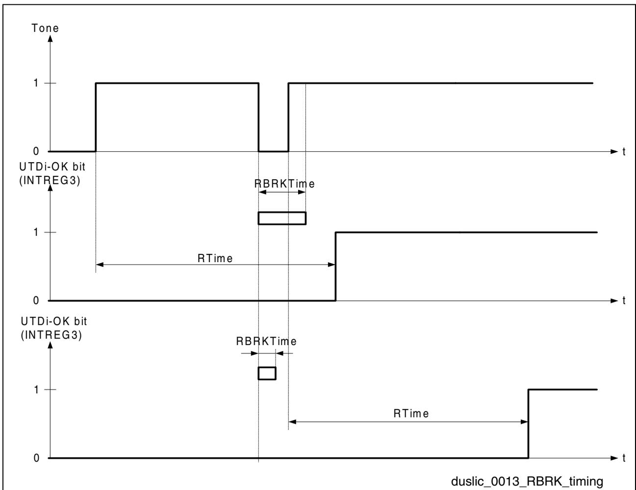
**Figure 64 Example for UTD Recognition Timing**
