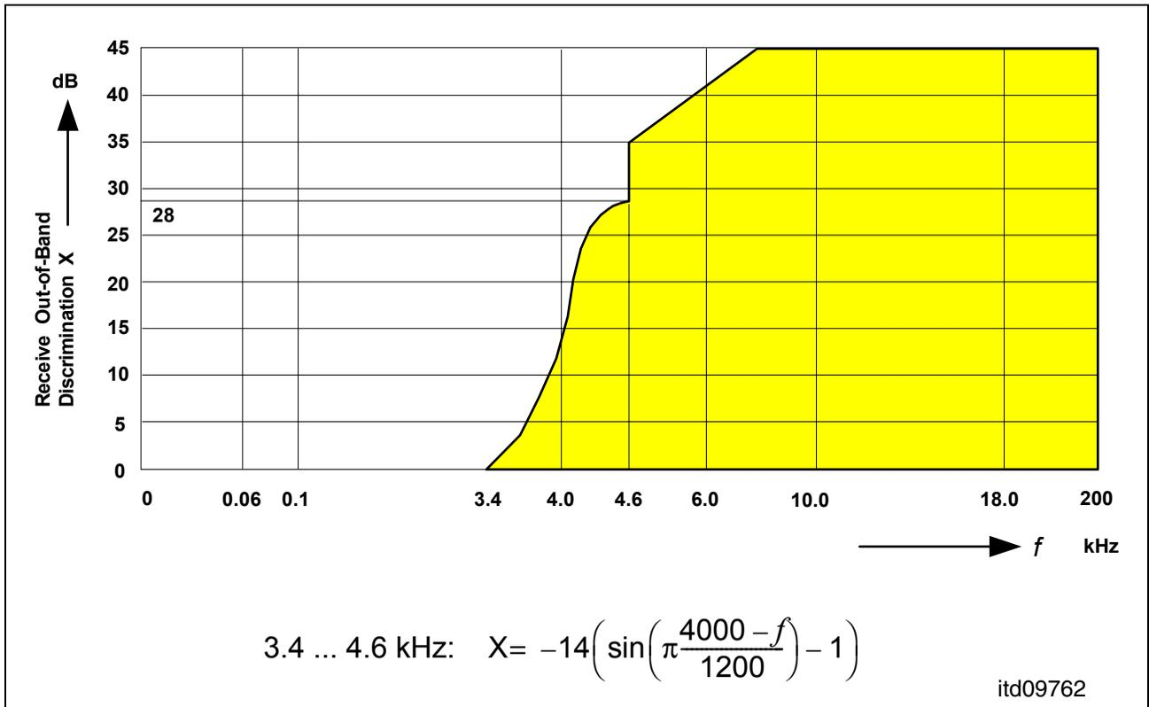
Figure 78 Out-of-Band Signals at Analog Output (Receive)
