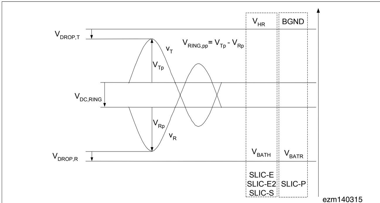
**Figure 24** Balanced Ringing via SLIC-E/-E2, SLIC-S and SLIC-P
