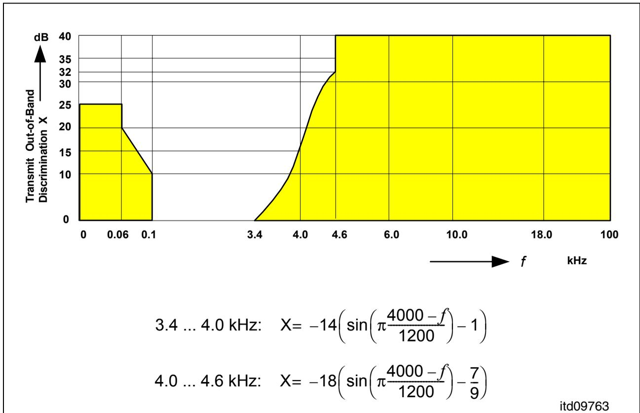
Figure 79 Out-of-Band Signals at Analog Input (Transmit)
