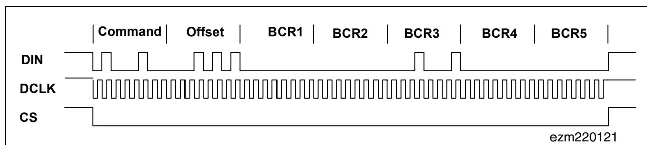
**Figure 66 Waveform of Programming Example SOP-Write to Channel 0**
