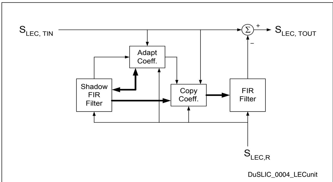
**Figure 31 Line Echo Cancellation Unit Block Diagram**
