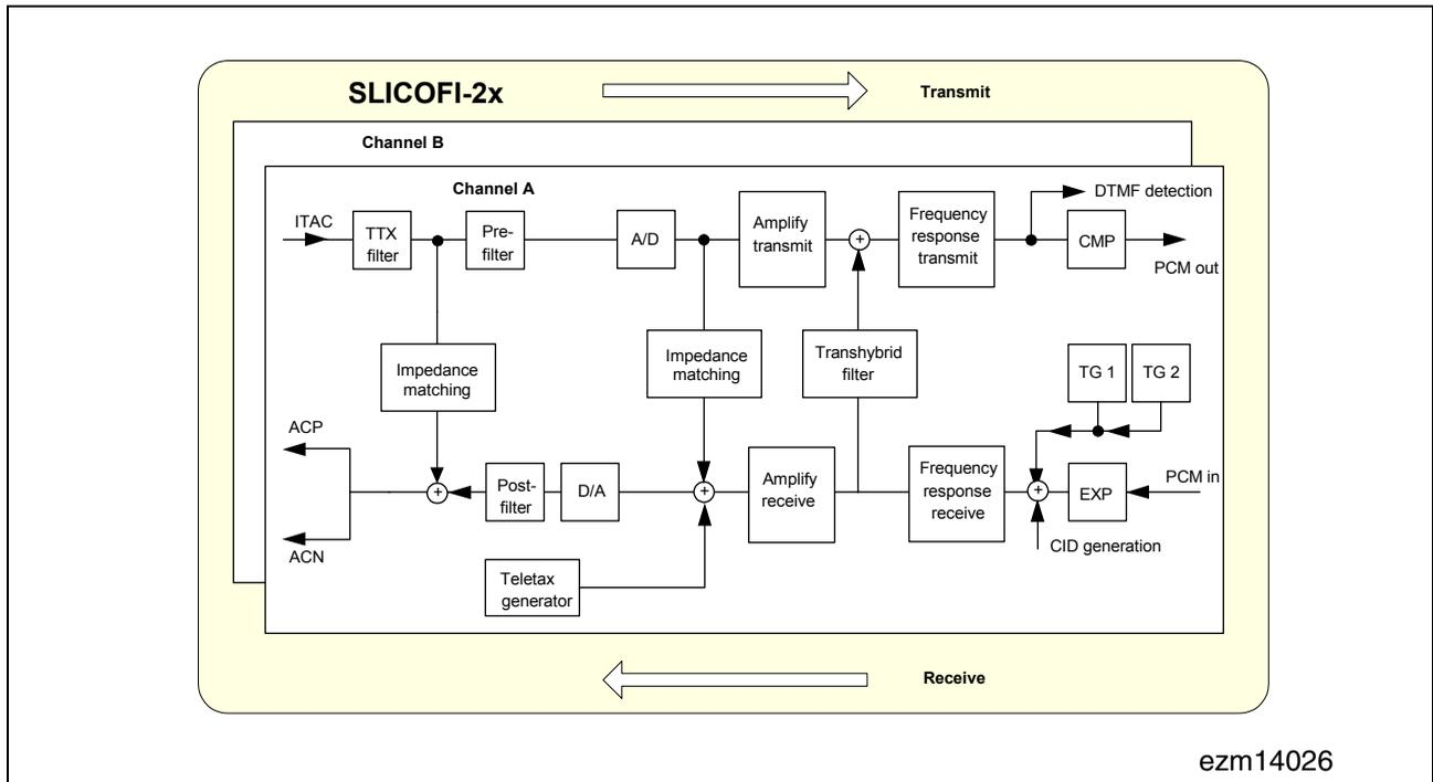
Figure 20 Signal Flow in Voice Channel (A)
