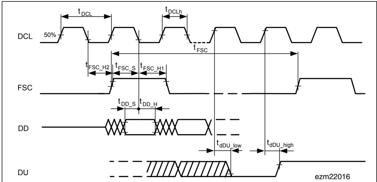
Figure 88 IOM-2 Interface Timing – Single-Clocking Mode
