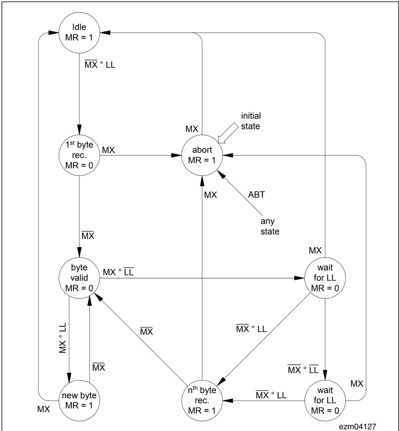
**Figure 61 State Diagram of the SLICOFI-2x Monitor Receiver**
