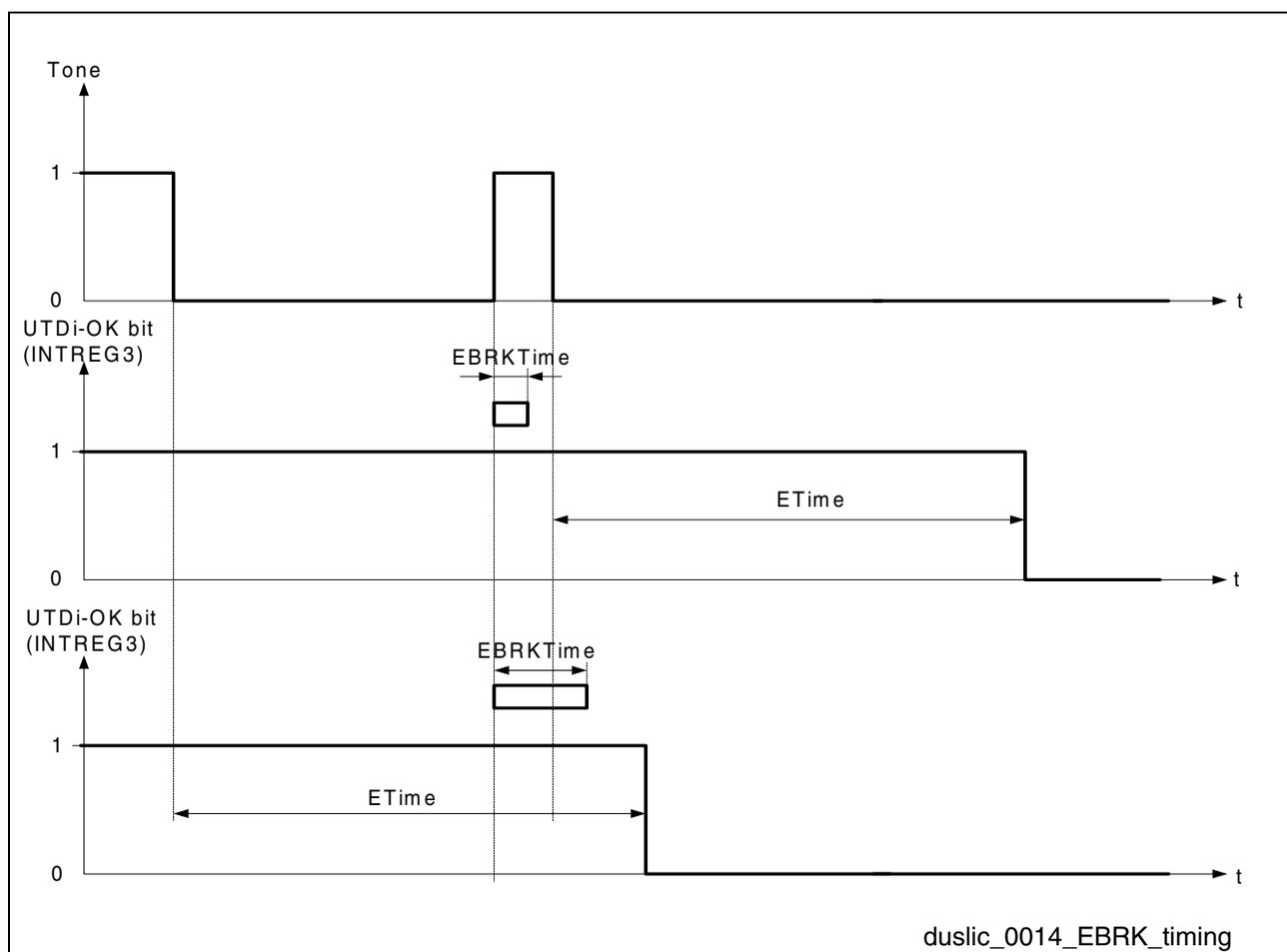
**Figure 65 Example for UTD Tone End Detection Timing**
