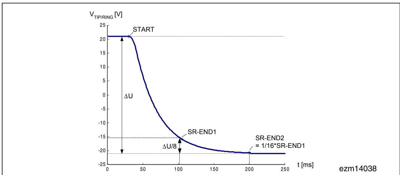
**Figure 27 Soft Reversal (Example for Open Loop)**
