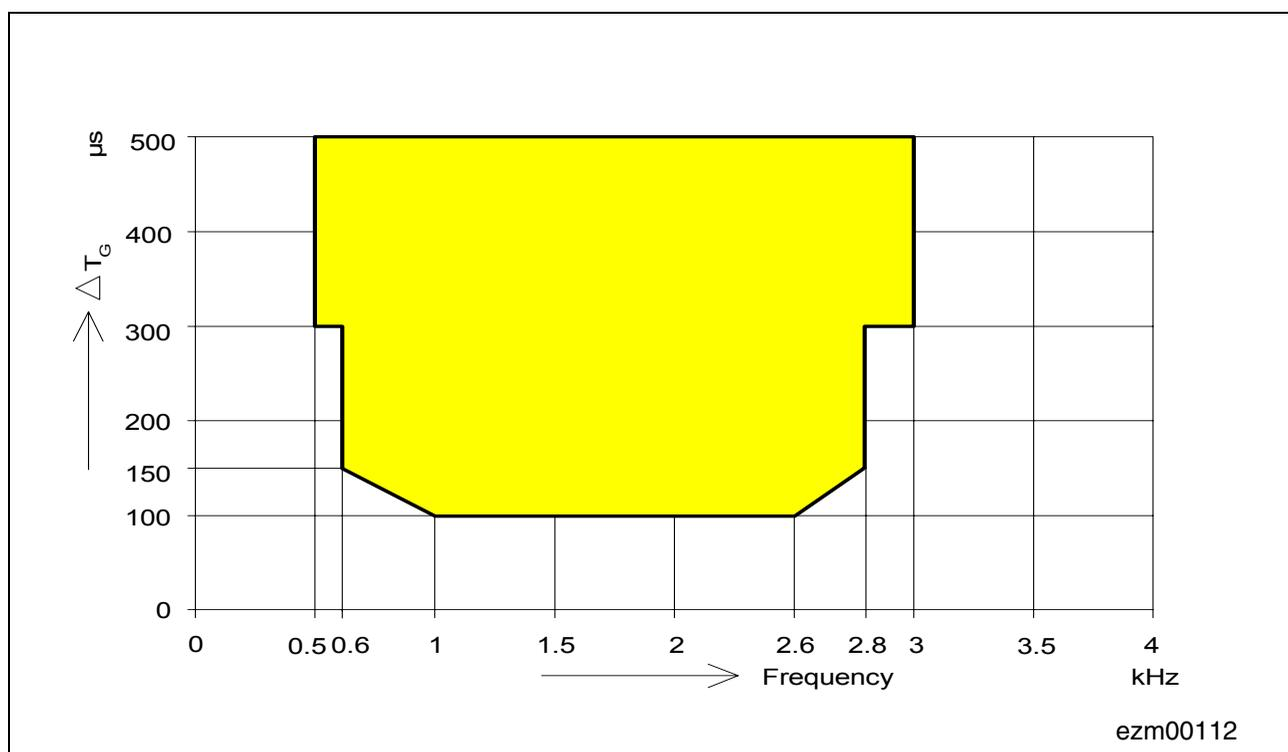
**Figure 77 Group Delay Distortion Receive and Transmit**
