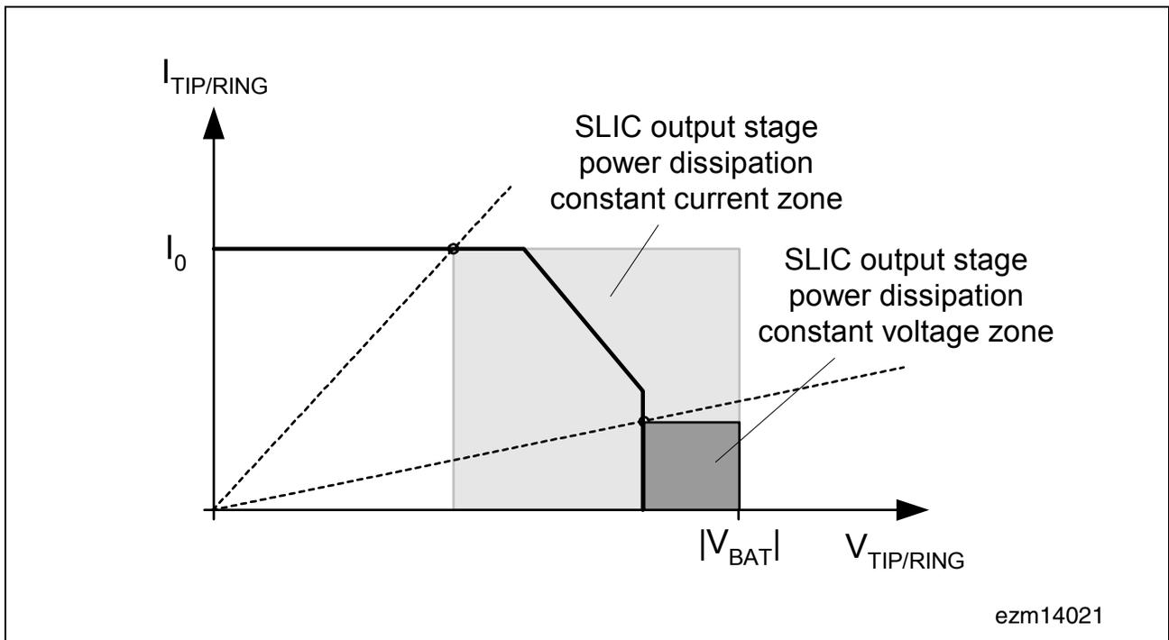
**Figure 16 Power Dissipation**
