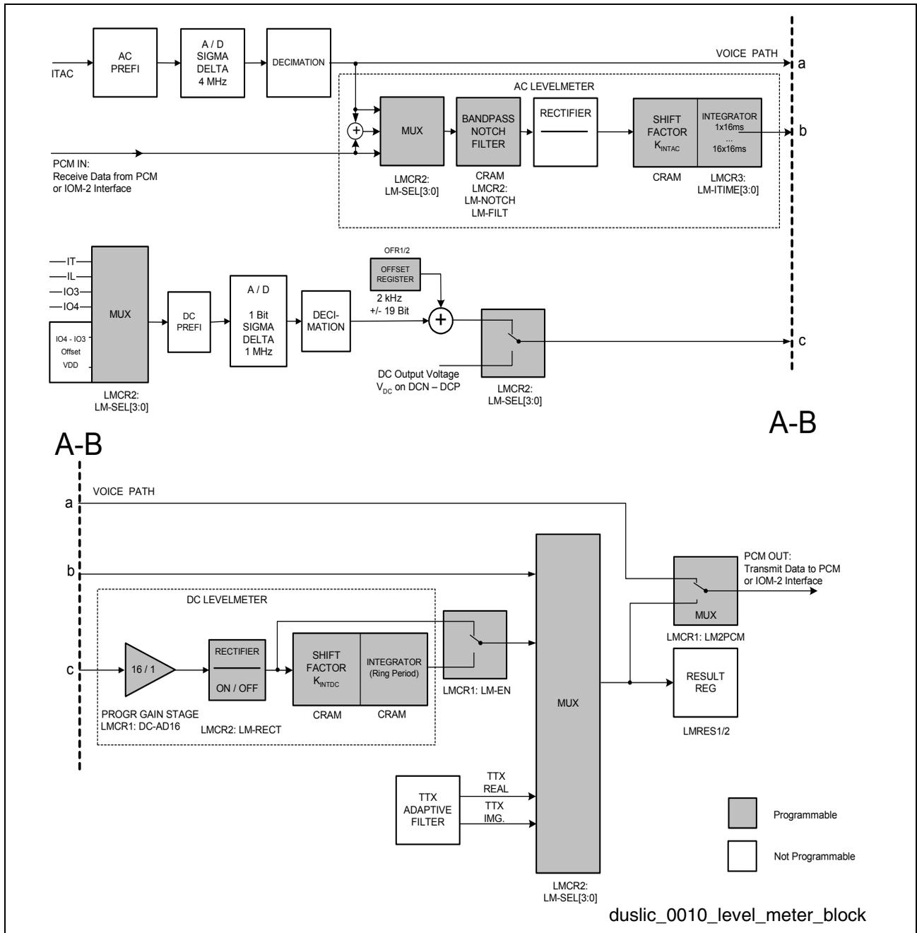
Figure 40 Level Metering Block Diagram
