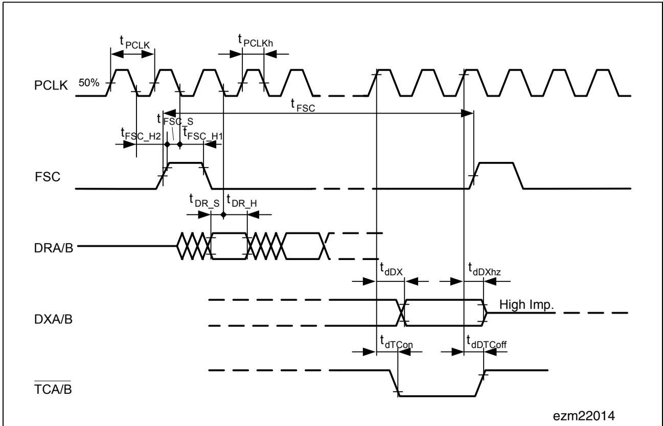
**Figure 86** PCM Interface Timing – Double-Clocking Mode
