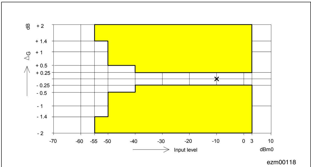
**Figure 76 Gain Tracking Transmit**
