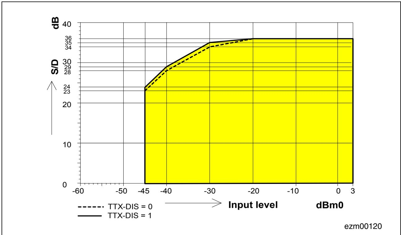
**Figure 82 Total Distortion Receive ( $L_R = 0$  dBr)**
