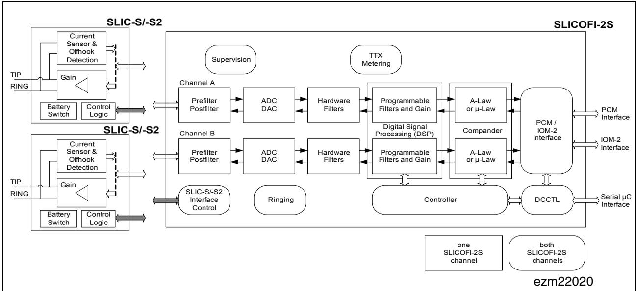
Figure 7 Line Circuit Functions in the DuSLIC-S/-S2
