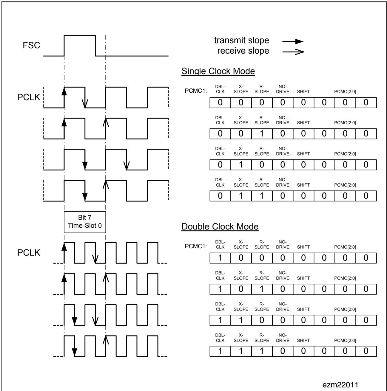
**Figure 53** Setting the Slopes in Register PCMC1
