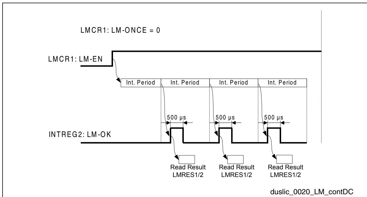
**Figure 42 Continuous Measurement Sequence (DC Level Metering)**
