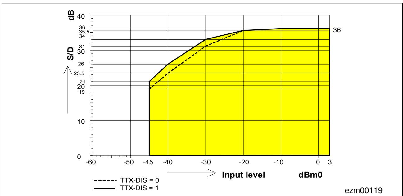
**Figure 81 Total Distortion Receive ( $L_R = -7$  dBr)**
