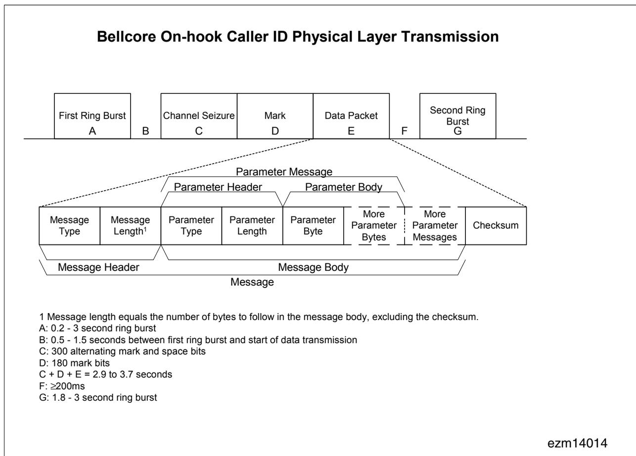
**Figure 30 Bellcore On-Hook Caller ID Physical Layer Transmission**
