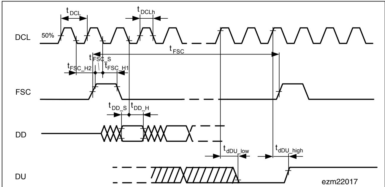
**Figure 89 IOM-2 Interface Timing – Double-Clocking Mode**
