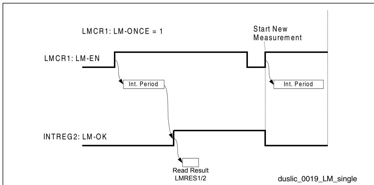
**Figure 41 Single Measurement Sequence (AC & DC Level Metering)**
