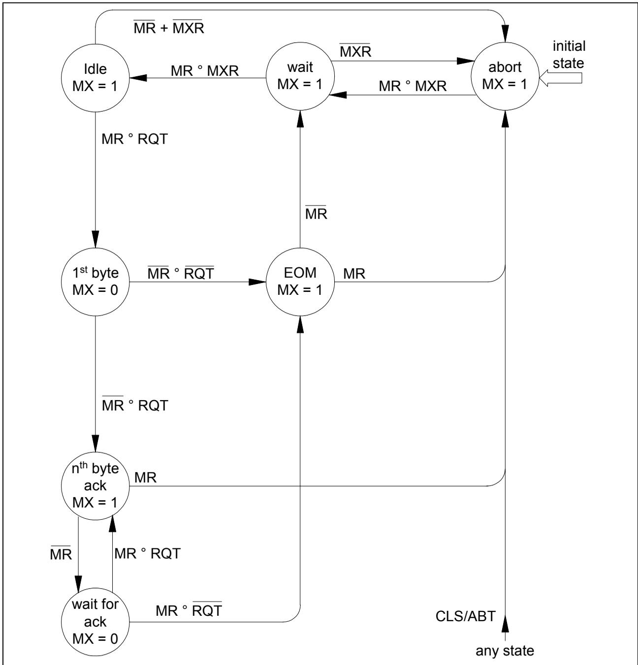
**Figure 60 State Diagram of the SLICOFI-2x Monitor Transmitter**
