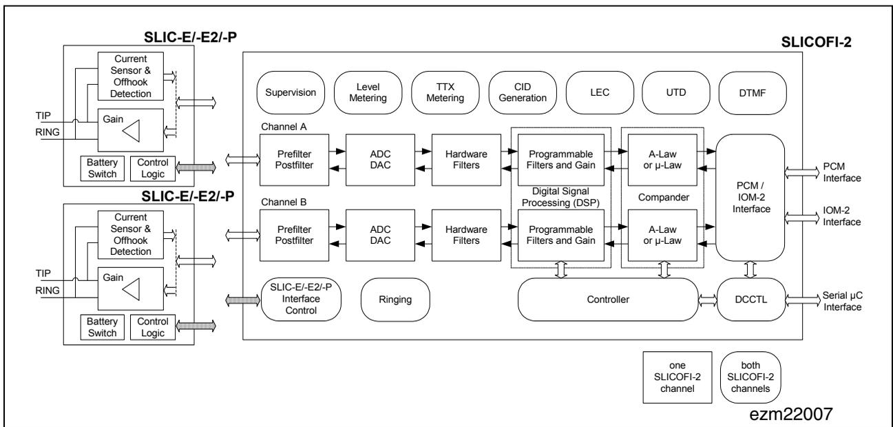
Figure 8 Line Circuit Functions in the DuSLIC-E/-E2/-P
