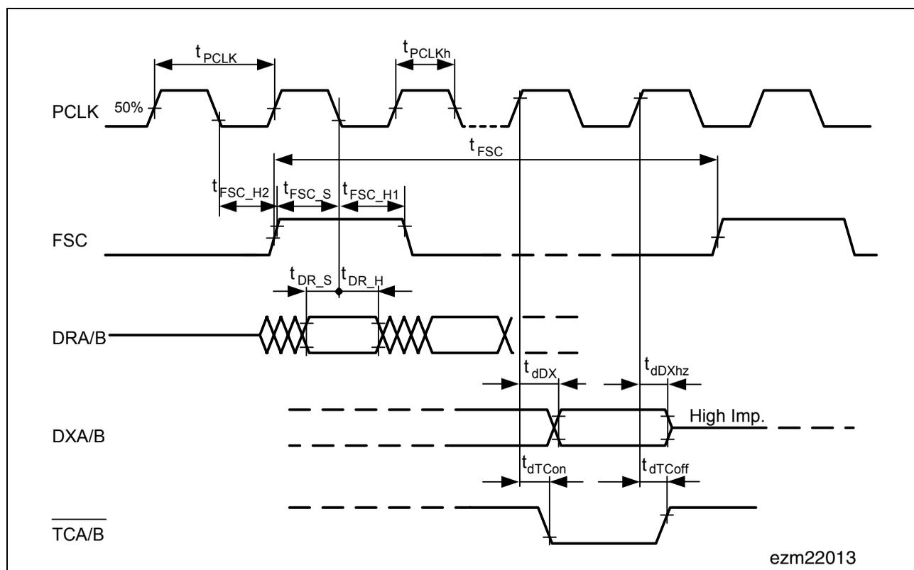
Figure 85 PCM Interface Timing – Single-Clocking Mode
