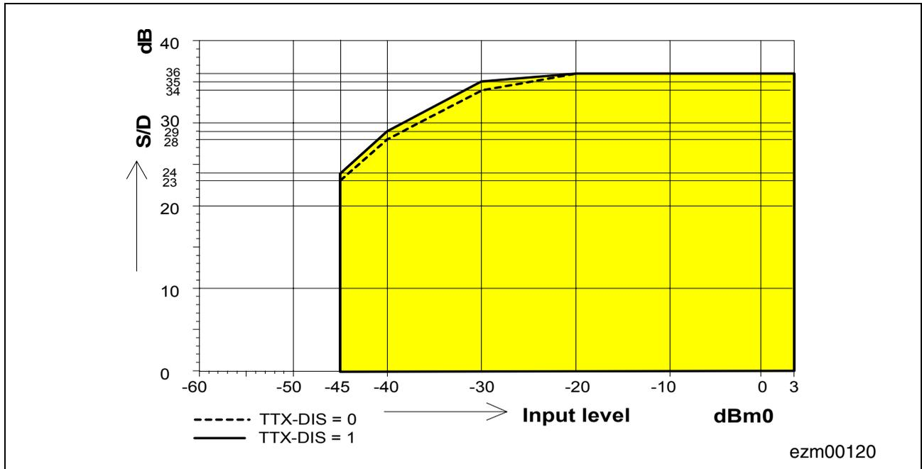
**Figure 80 Total Distortion Transmit ( $L_x = 0$  dBr)**
