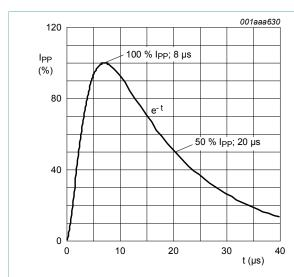
Fig. 1. 8/20 μs pulse waveform according to IEC 61000-4-5 and IEC 61643-321
