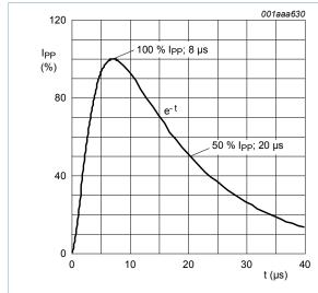
Fig. 2. 8/20 μs pulse waveform according to IEC 61000-4-5 and IEC 61643-321
