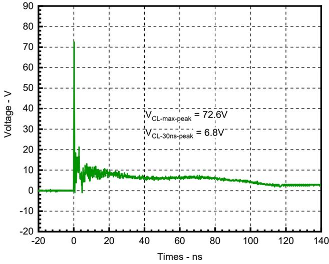
Fig 7. Clamping Voltage at IEC61000-4-2 +8kV Pulse Waveform
