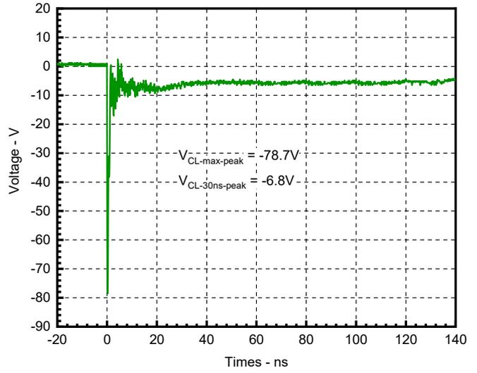
Fig 8. Clamping Voltage at IEC61000-4-2 -8kV Pulse Waveform
