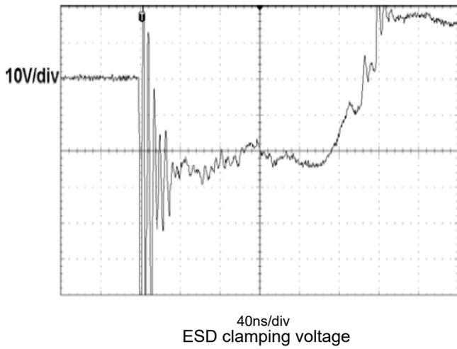
Fig 9. (IEC61000-4-2-8KV contact)
