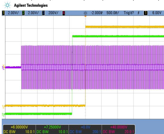
Figure 9: Turn-On AC Line 230 VAC, full load (5 ms/div)
