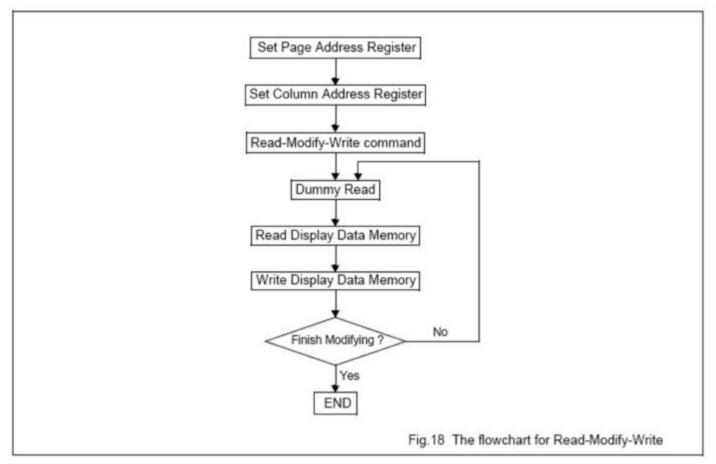
The setting of the control bus for the Read-Modify-Write command
