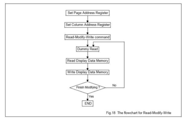
The setting of the control bus for the Read-Modify-Write command
