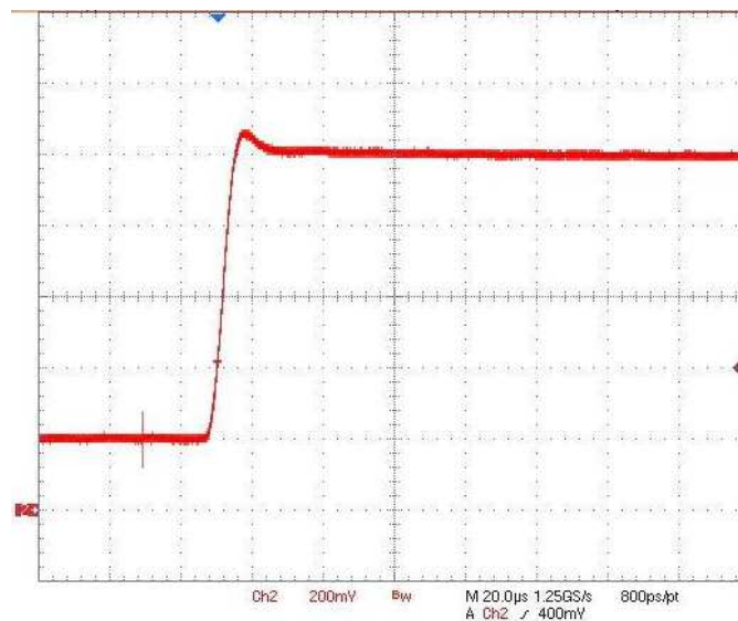
Figure 75. Loop Current Step From 4 mA to 20 mA
