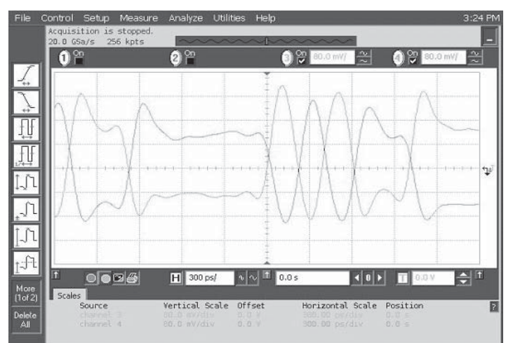
Data Waveforms, 2.5Gbps (left) & 5.0Gbps (right)
