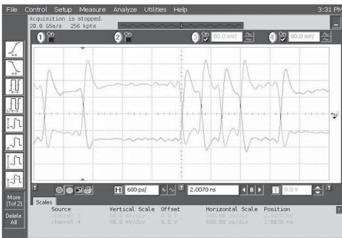
Data Waveforms, 2.5Gbps (left) & 5.0Gbps (right)
