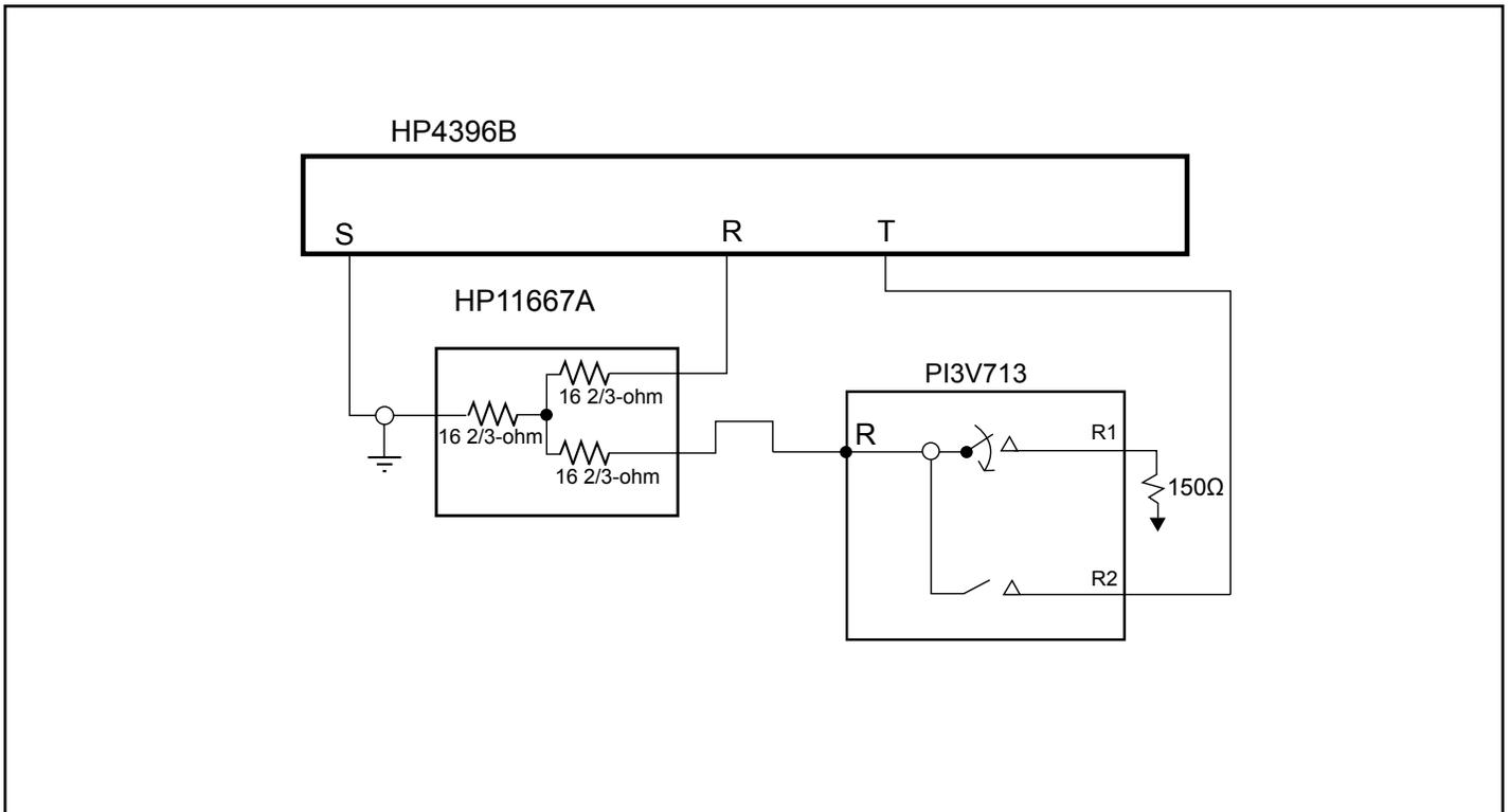
Figure 3. Off Isolation Test Setup
